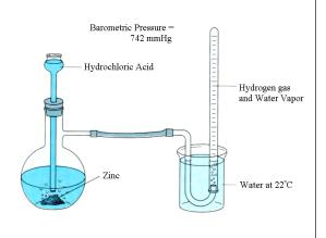
Inside the tube, both H<sub>2(g)</sub> and water vapor, H<sub>2</sub>O<sub>(a)</sub>, are present.
