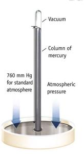
A barometer measures air pressure based on the height of a column of mercury it can support.
