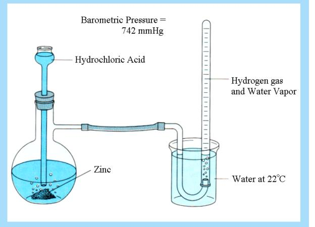
Inside the tube, both H<sub>2(g)</sub> and water vapor, H<sub>2</sub>O<sub>(g)</sub>, are present.
