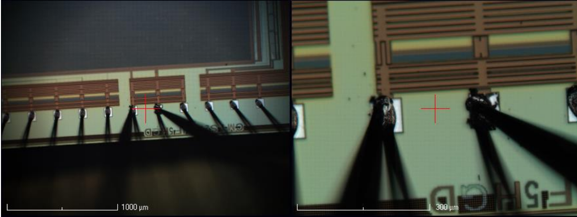
Figure 18. Power supply section of chip under test
