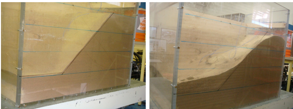
Figure 2: Left: Model slope before shaking with earthquake load; Right: Collapsed slope after shaking it with earthquake magnitude slightly higher than the Northridge Earthquake.
