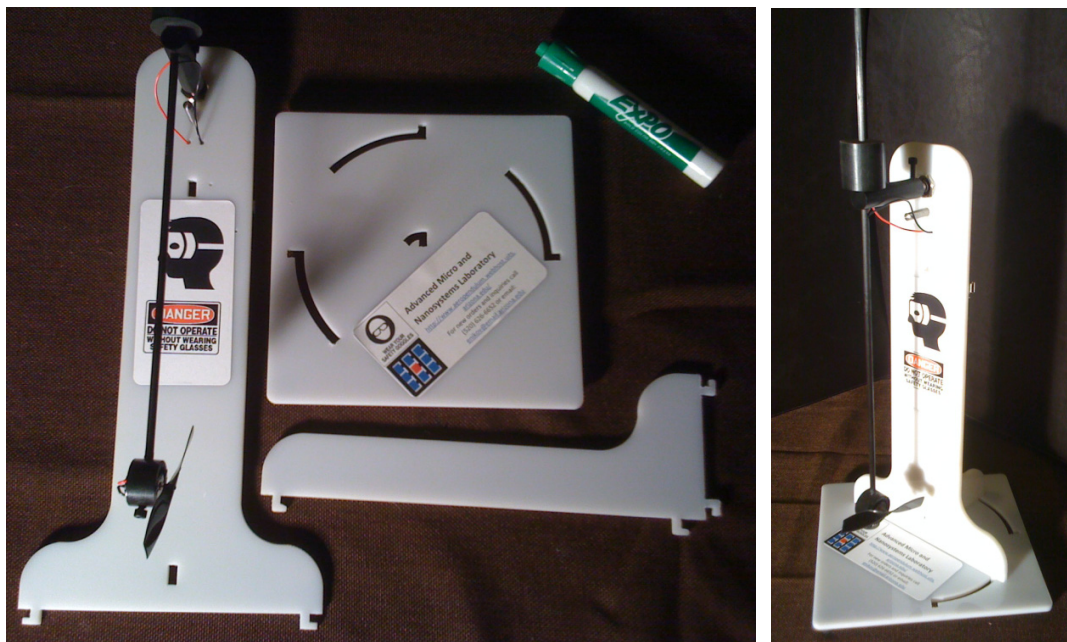
Figure 1. Aeropendulum Kit: Flat Configuration for During Shipping (left); Operating Configuration (right)
