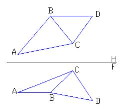
The top and front views of a three-dimensional truss ABCD are shown in the figure. Using appropriately selected auxiliary reference planes, construct auxiliary views that show the true length and slope angle of each of the lines AB and CD.
