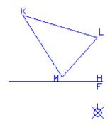
**Problem 3:** Find the piercing point of the line and plane by an auxiliary view off the top view. Show visibility of the line in all views.
