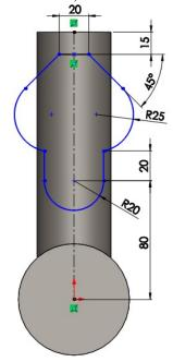
10. With the sketch fully defined, create a **Boss Extrude** feature of **70mm**. (*Hint: Notice in the image below that the feature is extruded in two directions*).
