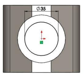
15. To create the cut-out, use an **Up to Surface** End Condition. In the Face/Plane Selection Window, select the face shown below.
