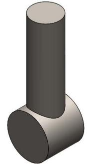
8. Next, create another extrude feature. Begin a sketch on the **Front Plane**, and sketch the following geometry. Then, use the Mirror Entities Sketch Tool (1) to mirror the geometry about the centerline.
