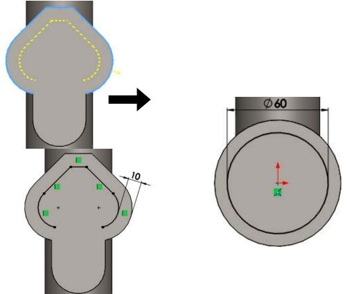
c. To finish the sketch, connect the two end-points with a line as shown to the right.
