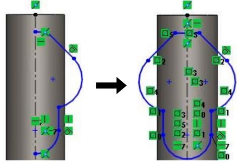
9. To fully define the sketch, dimension the sketch as shown below. (*Hint: To add the 10mm dimension, select the top of the cylinder, and while holding down the Shift Key, select the circle*).
