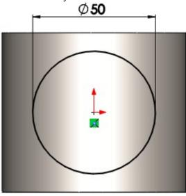
7. Create a **Boss Extrude**, and enter a **Blind Depth** of **180mm**.
