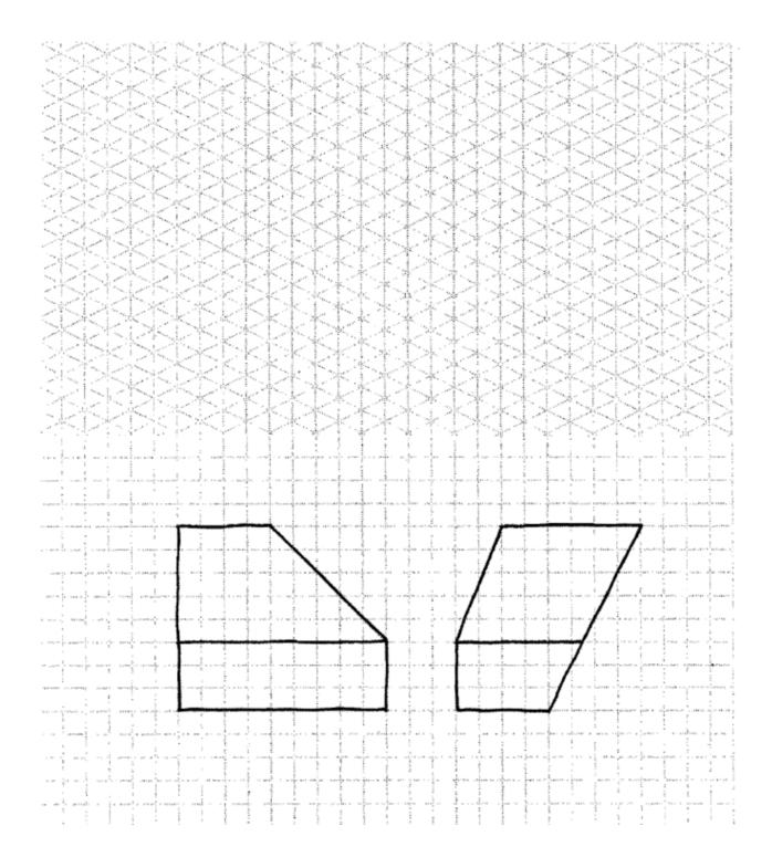
7.3 Create the missing top view. Then sketch an isometric view of the object.
