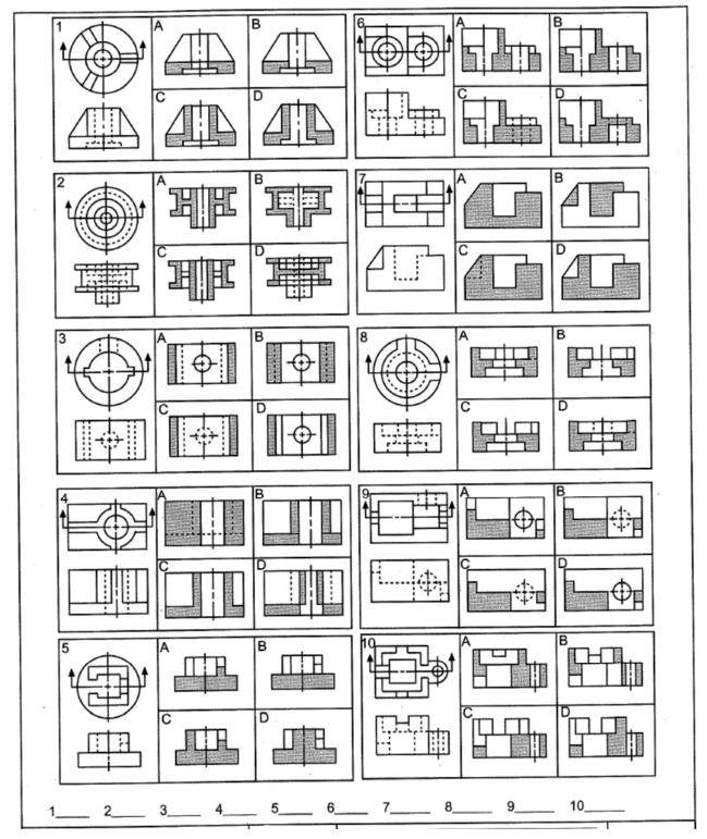
8.2 Section Views: Given the front view and a side view (either left or right), sketch the section view as indicated by the cutting plane line. Hint: You need to rotate this page 90° clockwise before you start your drawings.
