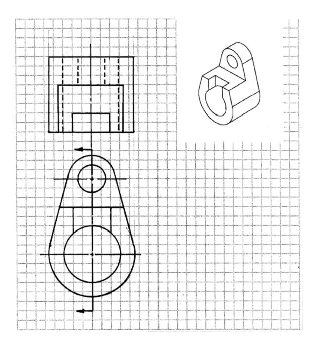
2. Sketch the Right Side section view as determined by the cutting plane.
