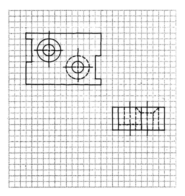
4. Create a cutting plane on the Front View through the counterbore and then sketch the resultant Right Side section view.
